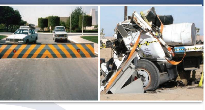
offer maximum security against military sites and airports. elkosta at 80 km/h. The very first impact unauthorized vehicles of all sizes Road Blockers DSP® K12 are test was conducted by the TÜV and weights for highly sensitive designed to guarantee the full level (German Technical Inspectorate) entry points. of application are: embassies, crash tested according to DOS SD-
